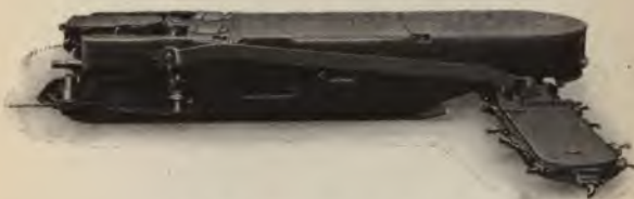
Arm in Position for Running Cut
